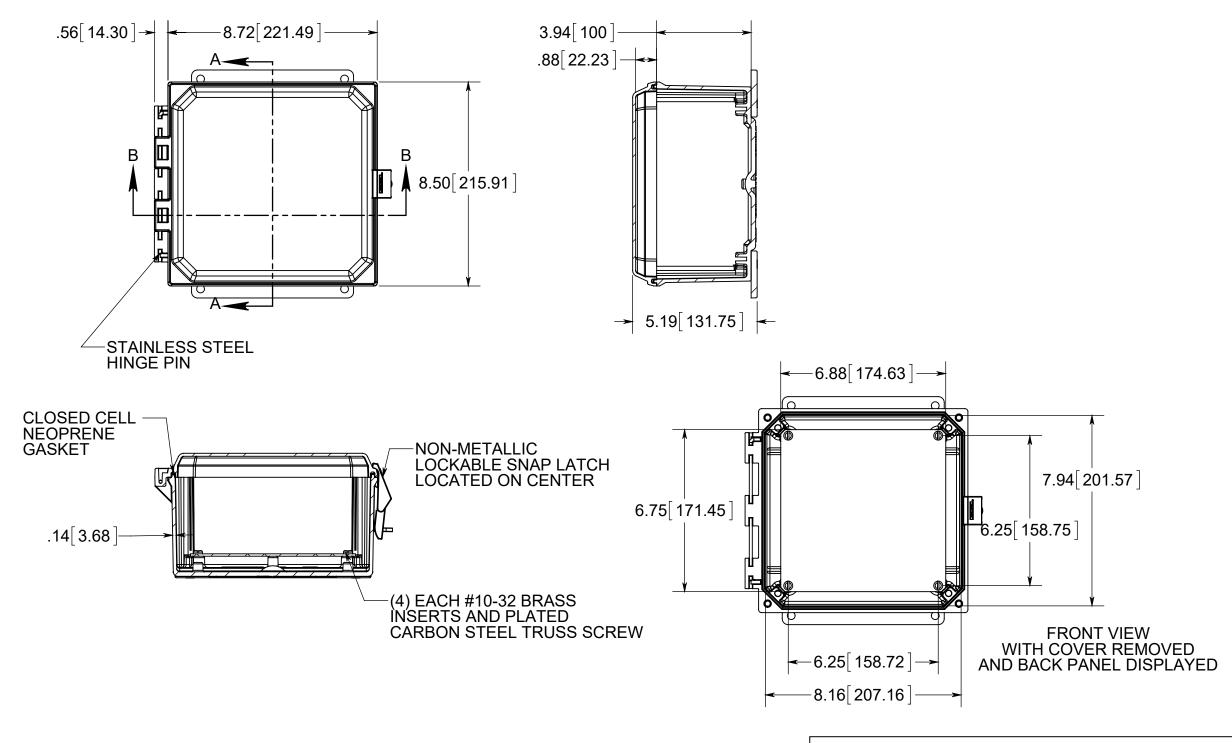
MATERIAL: BOX - INJECTED POLYCARBONATE COVER - INJECTED POLYCARBONATE
