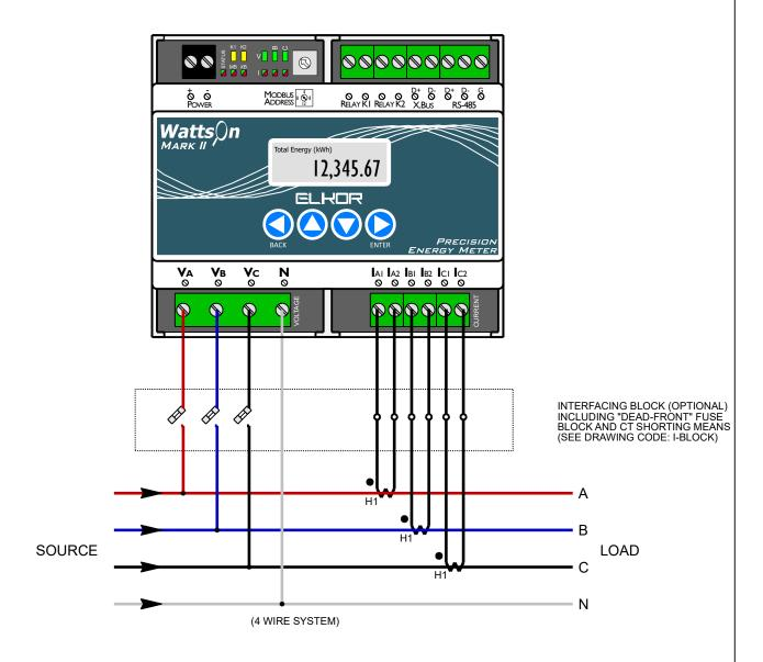
WIRING USING STANDARD 5A CTs SHOWN. WHEN USING 5A CTs, ELKOR RECOMMENDS THE USE OF A SHORTING BLOCK.
