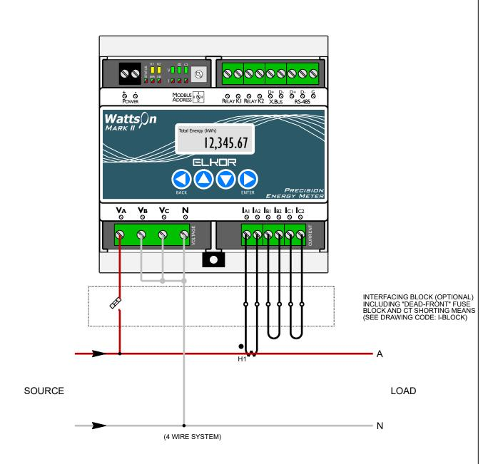
WIRING USING STANDARD 5A CTs SHOWN. WHEN USING 5A CTs, ELKOR RECOMMENDS THE USE OF A SHORTING BLOCK.
