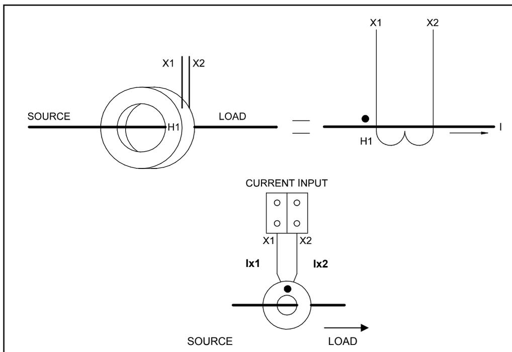
Note: Usually, CTs are marked as shown above, where the 'H1' indicates the primary current input and 'X1' the corresponding secondary current terminal (or lead).
