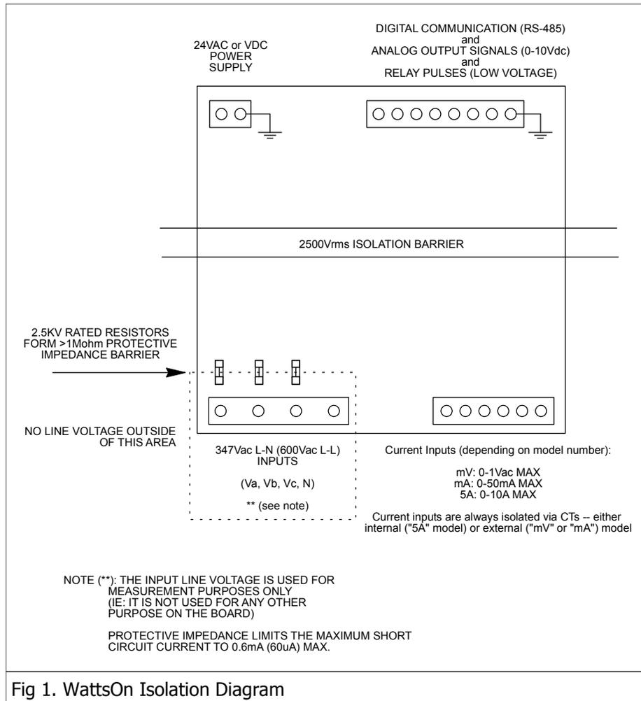
Fig 1. WattsOn Isolation Diagram
