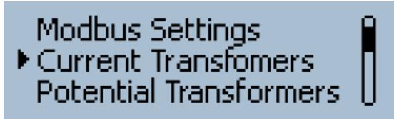
Pressing the Up / Down buttons moves the cursor to the next and previous menu items, respectively, and pressing the Forward / Enter button confirms the selection. Some menu items bring up sub-menus; pressing the Back/Menu button, leaves a sub-menu to go back to the previous menu.
